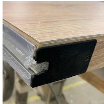
Lock edge installed
