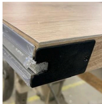
Lock edge installed
